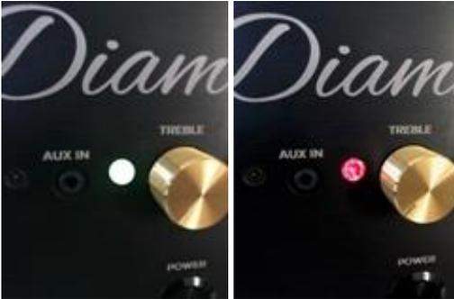
If audio quits playing and the Diamond is RED mixed with a flashing pink/blue color this means the battery is completely discharged and music has been muted to protect it from further discharge. If this happens please plug charger into DiamondBoxx and let charge for a few minutes before expecting the DiamondBoxx to unmute and start playing music again.
