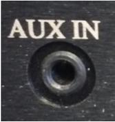
The front panel AUX IN jack has ZERO LATENCY and can be connected to just about anything with an audio output. This would include:
