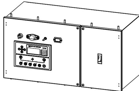
PLC-7420 is an advanced control module based on micro-processor, containing all necessary functions for protection of the genset and the breaker control. It can monitor the mains supply, and automatically start the engine when the mains is abnormal. Accurately measure various operational parameters and display all values and alarms information on the LCD. In addition, the control module can automatically shut down the engine and indicate the engine failure.
