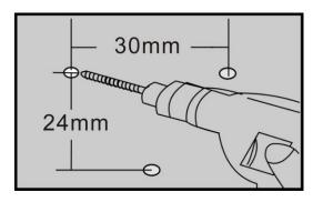
2. Insert plastic raw plugs into the three holes.
