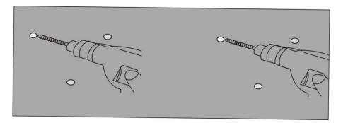
2. Insert plastic raw plugs into the six holes.
