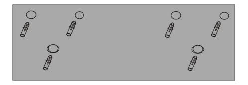
3. Fix the bracket into place by using the six ST4\*35 screws and make sure the it is fixed securely.
