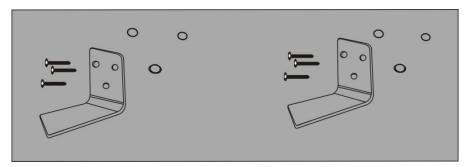
4. Before attaching the heater, make sure the power switch is on. Fix the heater onto the bracket using the four M6\*14 screws and butterfly nuts
