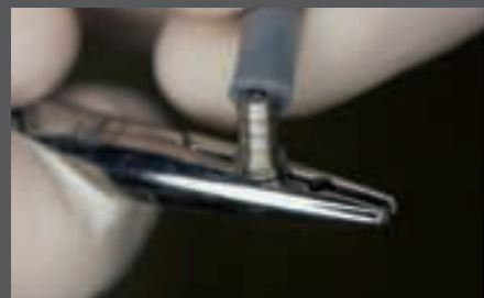
To insert new tube hold the tube with right index finger and thumb close to the fitting, with up-down movement push the tube in position
