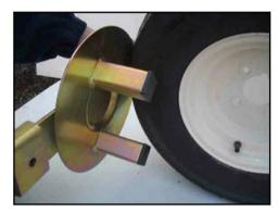
1. With the tyre valve positioned away from the tubes welded to the inside of the Trail Clamp disc, hook the arm behind the wheel.
