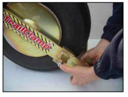
3. With the lock in the unlocked position, slide the return arm in around the rear of the tyre and lock by pressing the plunge lock in until it clicks.
