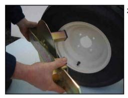
2. With the arm hooked behind the wheel, move the arm of the Trail Clamp in So that it lies flat against the tyre.
