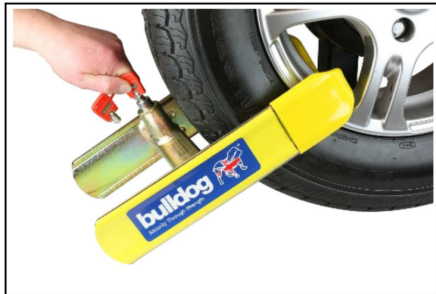
4. To remove clamp, insert key, rotate 1/2 turn, pull on key and/or press inner and outer arms together until lock pops out.
