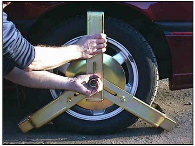
7. Still holding nut with left hand, swing round top arm to vertical position.
