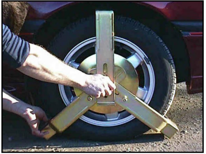
9. At this point hold up nut with right hand and pull left wheel clamp arm in tightly to tyre. Now hand tighten nut.
