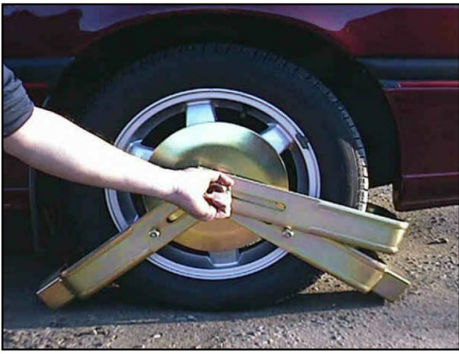
6. With left hand lift nut and disc assembly to centre wheel.
