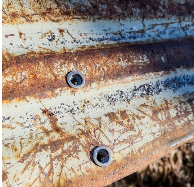
Figure 1: Rivnuts installed in tailgate. For this spoiler the rivnuts need to be on the raised stamping on the tailgate.
