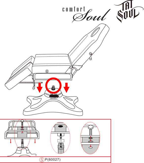
Step5. Place Seat Frame Bracket on to lift piston, aligning seat frame notch with piston peg. Then Fasten Seat Frame Bracket to Lift Piston, using bolt with washer and gasket.
