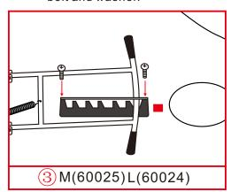
Step3. Insert Back Adjustment Bar into Back Teeth, then fasten back teeth cover bar over top with cross bar mounting screws.
