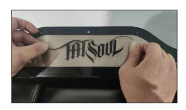
Step 3: With a hard lined tool, such as a squeegee, apply even pressure over the sticker to transfer it.
