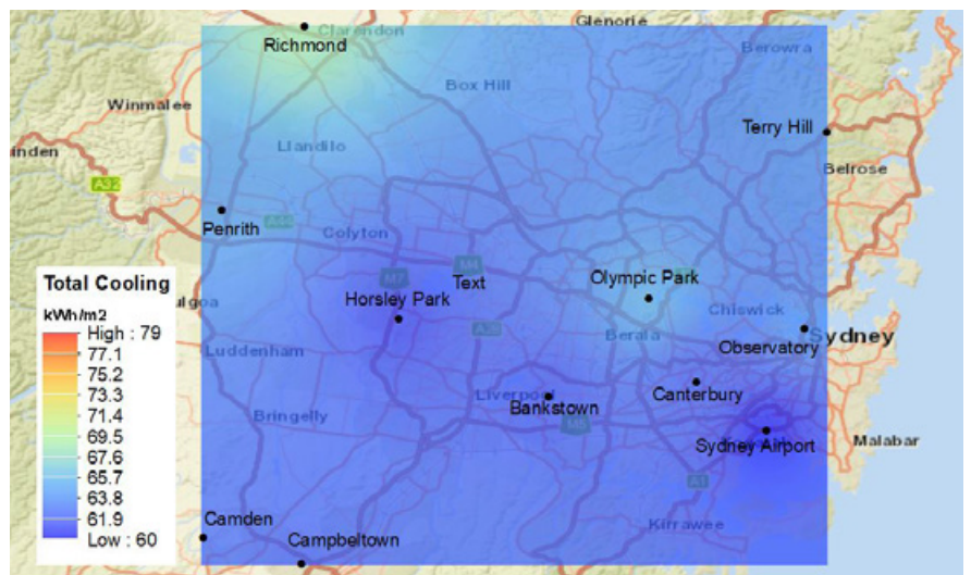
Figure 3. Spatial distribution of total cooling load for cool roof with modified urban temperature scenario (scenario 2) for two summer months (i.e. January and February) for an existing high-rise shopping mall centre with weather data simulated by WRF for COP=1 for heating and cooling.
