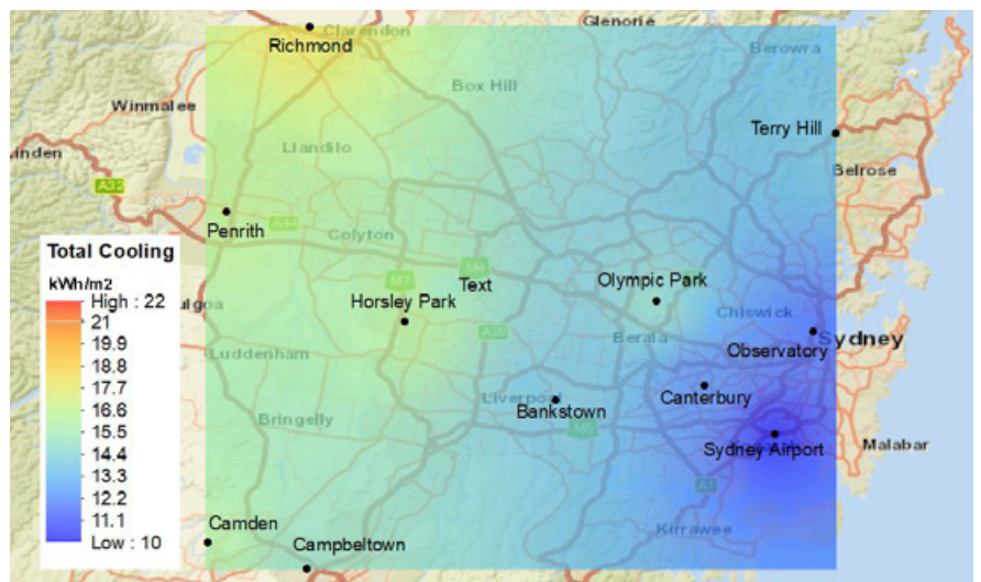
Figure 3. Spatial distribution of total cooling load for cool roof with modified urban temperature scenario (scenario 2) for two summer months (i.e. January and February) for an existing low-rise office building with roof insulation with weather data simulated by WRF for COP=1 for heating and cooling.
