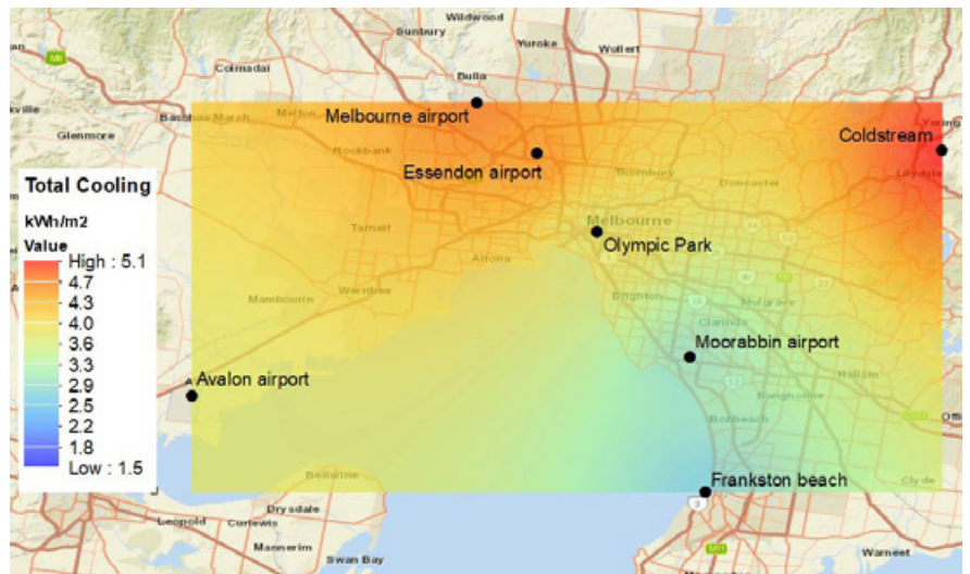
Figure 2. Spatial distribution of total cooling load for reference with cool roof scenario (scenario 1) for two summer months (i.e. January and February) for a new low-rise apartment building with weather data simulated by WRF for COP=1 for heating and cooling.
