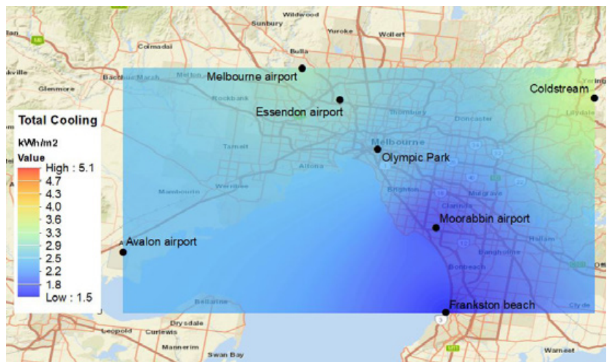
Figure 3. Spatial distribution of total cooling load for cool roof with modified urban temperature scenario (scenario 2) for two summer months (i.e. January and February) for a new high-rise apartment building with weather data simulated by WRF for COP=1 for heating and cooling.
