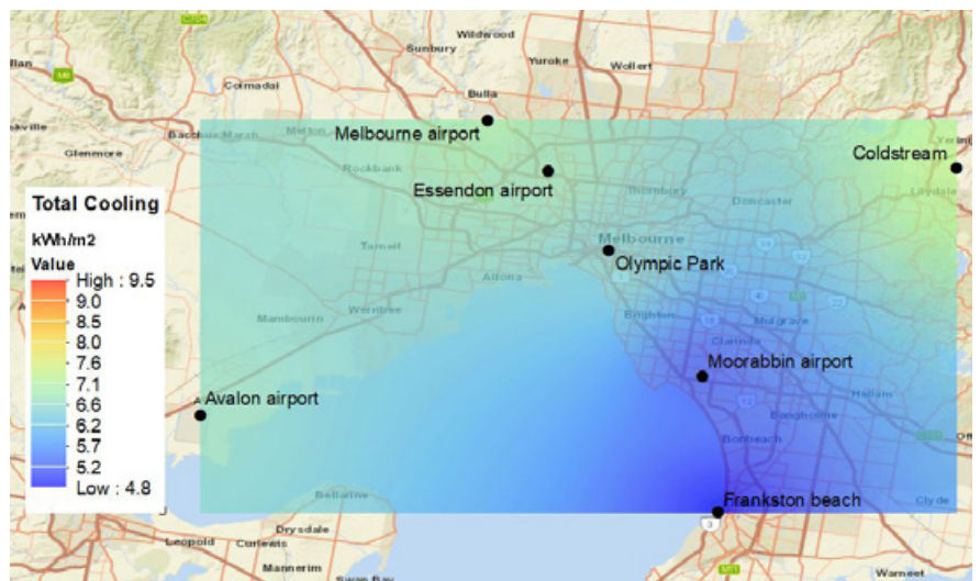
Figure 3. Spatial distribution of total cooling load for cool roof with modified urban temperature scenario (scenario 2) for two summer months (i.e. January and February) for a new low-rise office building with roof insulation with weather data simulated by WRF for COP=1 for heating and cooling.
