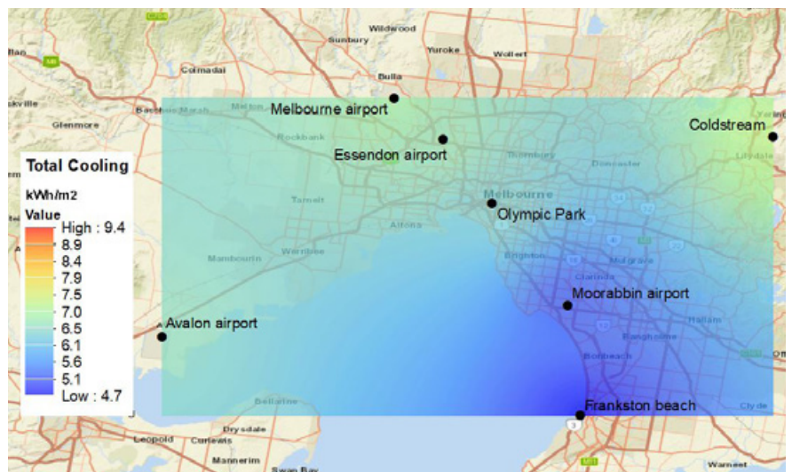
Figure 3. Spatial distribution of total cooling load for cool roof with modified urban temperature scenario (scenario 2) for two summer months (i.e. January and February) for an existing high-rise office building with insulation with weather data simulated by WRF for COP=1 for heating and cooling.
