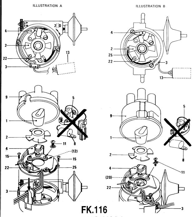
Lucas 22, 23 & 25D 4 & 6 Cylinder Distributors. Anti-Clockwise Rotor Rotation
