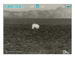
**NOTE:** A red warning icon ① appears next to the camera icon in the upper-right corner of the screen when insufficient memory storage is available. Transfer video and image files to other storage media to free up space on the memory card.
