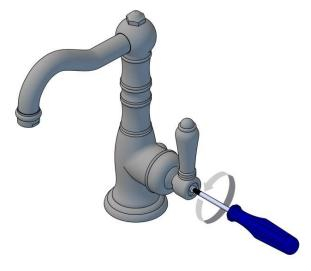
Hand loosen the retaining flange A .
