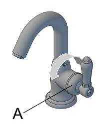
Once the retaining screw is loose, simply remove the handle and retaining flange.
