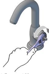
Once the cartridge nut is loose; simply remove the cartridge by pulling it from cartridge seating position.
