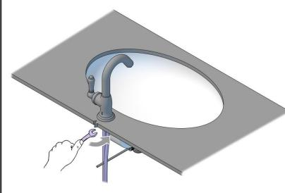
Connect hot and cold water supplies to the flexi tail hoses.
