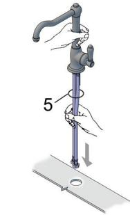
Check the position of the tap on the sink, then tighten the nut using a 13mm wrench.
