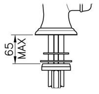
Install the water supply hoses 2, into the tap body -1
