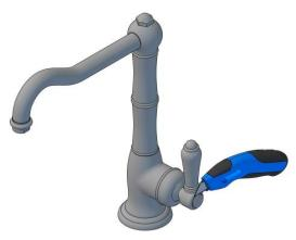
Unscrew the retaining screw with a Phillips head screw driver.
