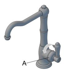
Once the retaining screw is loose, simply remove the handle and retaining flange.
