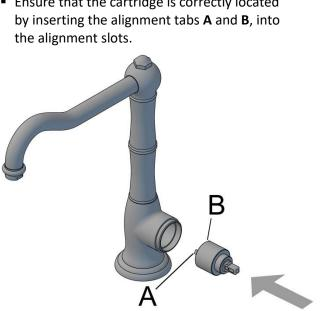
Once the cartridge nut is loose; simply remove the cartridge by pulling it from cartridge seating position.
