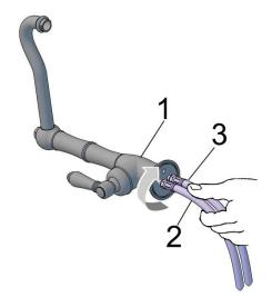
Install the 200mm hand spray water supply hose 3, into the tap body - 1
