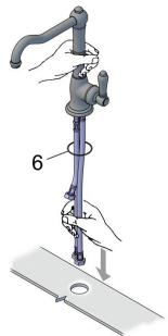
• Check the position or the tap on the sink, then tighten the nut using a 13mm wrench.
