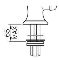
Install the hot and cold water supply hoses 2 and 3, into the tap body -1
