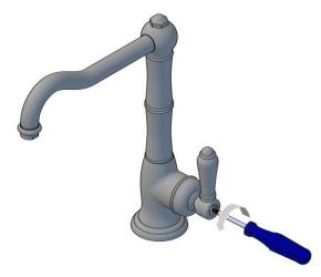
Once the retaining screw is loose, simply remove the handle and retaining flange.
