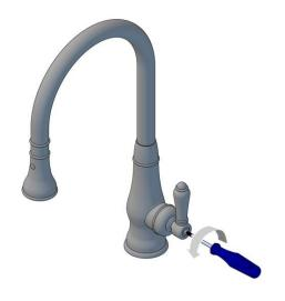
Hand loosen the retaining flange A .
