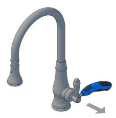
Unscrew the retaining screw with a Phillips head screw driver.
