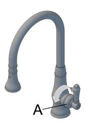
Once the retaining screw is loose, simply remove the handle and retaining flange.
