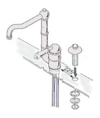
Insert the hand spray escutcheon into the sink hole
