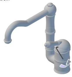
Lift the handle and carefully remove the dome from the cartridge lever arm.
