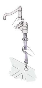
Insert the tap into mounting hole. Feed the water supply hoses carefully through the hole ensuring that they are not bent or kinked, as this could result in permanent damage or leakage.
