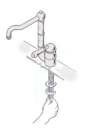
Under the sink, stack the supplied half ring rubber gasket above the half ring mounting plate and feed them onto the stud. Then screw the mounting nut onto the stud. Screw the mounting stud until the half ring rubber mates up with the underside of the
