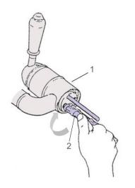
Install the water supply hoses into the body - 1
