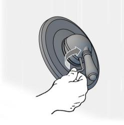
Install the indice button 9, into the access hole, and ensure that it is firmly pressed into position.
