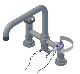
**Note:** Do not over tighten as this could damage the ceramic cartridge!
