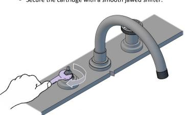
**Note:** Do not over tighten as this could damage the ceramic
