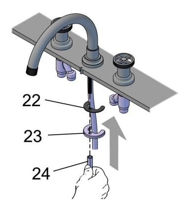
• Check the position on the spout body, then tighten the nut using a 13mm spanner or smooth jawed shifter.
