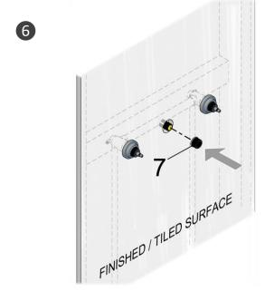
■ Fit the supplied ¾" to ½"adptor 7, into the thread section of the wall breech. Ensure it is properly sealed using PTFE tape or equivalent sealer to prevent any leakage.
