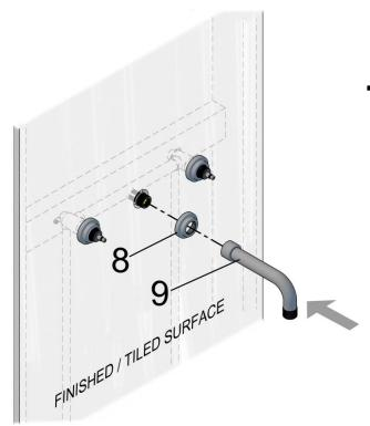
Place the cover plate 8, over the ¾" to ½"adptor. Line-up the thread end of the spout 9, with the thread of the adaptor. Apply the spout onto the adaptor and screw on until it is firmly secured. Ensure to apply adequate PTFE tape, or a suitable sealing material to the threads to prevent any leakage from the wall spout.
