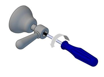
Once the retaining screw is loose, lift and remove the handle B, from cartridge spline
