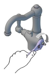
Note: Do not over tighten as this could damage the ceramic cartridge!
