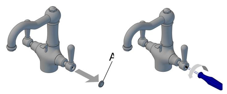
Once the retaining screw is loose, lift and remove the handle B, from cartridge spline.
