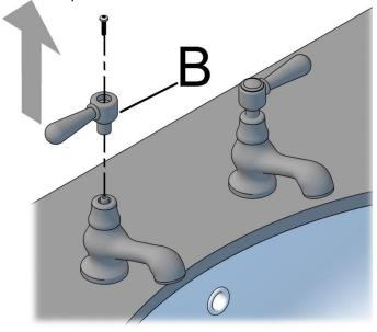
Using a Philips head screw driver, unscrew the handle retaining screw.
