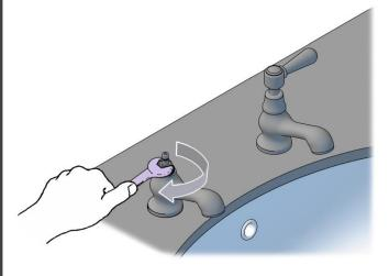
**Note:** Do not over tighten as this could damage the ceramic cartridge!
