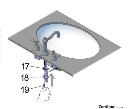
Check the position on the sink of the tap, then tighten the nut using a 13mm spanner or smooth jawed shifter.
