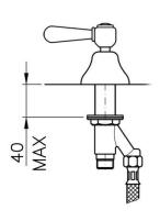
Measure and cut tap holes, with a minimum hole spacing of 110mm from tap body centre line.
