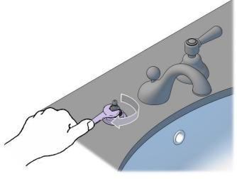
**Note:** Do not over tighten as this could damage the ceramic cartridge!
