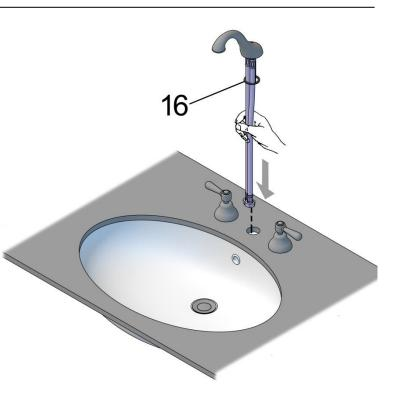
Check the position on the sink of the tap, then tighten the nut using a 13mm spanner or smooth jawed shifter.
