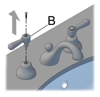
Using a Philips head screw driver, unscrew the handle retaining screw.
