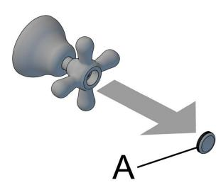
Using a Philips head screw driver, unscrew the handle retaining screw.
