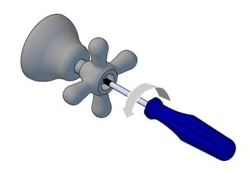
Once the retaining screw is loose, lift and remove the handle **B**, from cartridge spline.
