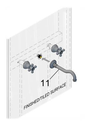
Line-up the spout 11, with the thread section of the wall breech. Screw the spout until it is firmly secured on the wall breech. Ensure to use adequate PTFE tape, or a suitable sealing material is applied the threads, to prevent any leakage from the wall spout.
