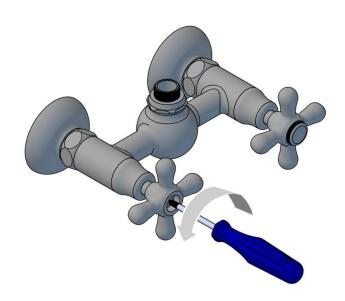
Once the retaining screw is loose, lift and remove the handle B, from cartridge spline.
