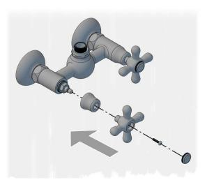
**Note:** Do not over tighten as this could damage the ceramic cartridge!
