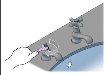
Remove the cartridge with a 17mm spanner or smooth jawed shifter.
