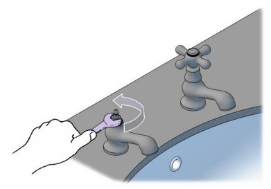
Install the tap handle and tap cover cap. Refer to "Removing and replacing a handle" section, page7, for additional information.
