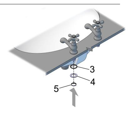
Check the and alignment or desired position of the tap spout, then tighten the nut using a smooth jawed shifter.
