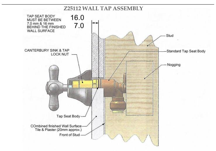
• A small amount of silicon can be applied behind the flange to hold it in place.
