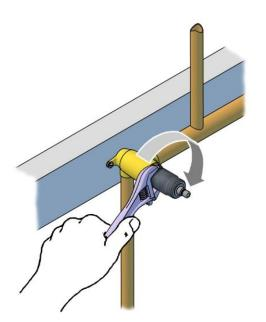
Fit the tap cover cap 5, onto the locknut outer thread.
