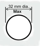
Measure and cut tap holes, with a minimum hole spacing of 110mm from tap body centre line.
