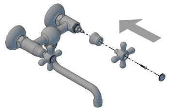
Note: Do not over tighten as this could damage the ceramic cartridge!
