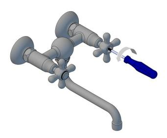
Once the retaining screw is loose, lift and remove the handle B, from cartridge spline.
