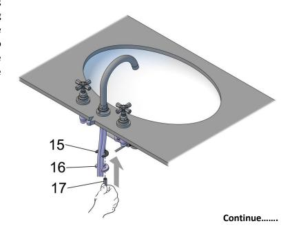
Check the position on the sink of the tap, then tighten the nut using a 13mm spanner or smooth jawed shifter.
