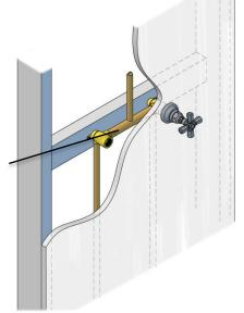
Install the C-tech ¼ turn cartridge 1, into the breech seat 2. Ensure that the base of the cartridge is firmly tightened onto the base of the seat.
