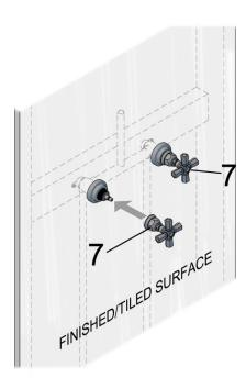
Position the retaining flange with Lever handle 7, over the cartridge shaft spline, and carefully hand turn the retaining flange onto thread until it is firmly seated.
