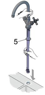
• Check the position of the tap on the sink, then tighten the nut using a 13mm wrench.
