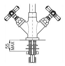
Install the water supply hoses 2, into the tap body -1
