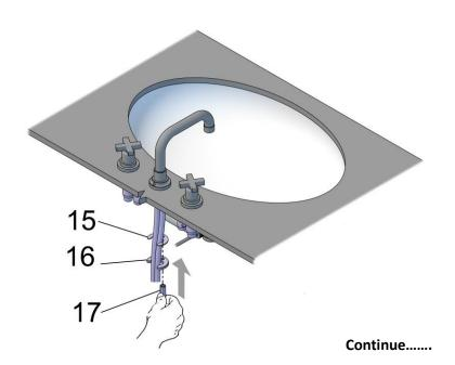
Check the position on the sink of the tap, then tighten the nut using a 13mm spanner or smooth jawed shifter.
