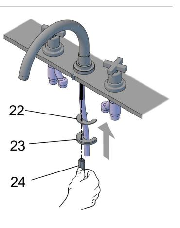
Check the position on the spout body, then tighten the nut using a 13mm spanner or smooth jawed shifter.
