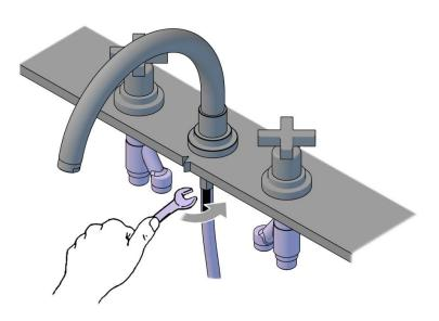
Connect main Hot and Cold water supplies to the Tap side body thread sections, using the correct flexi tail hoses.
