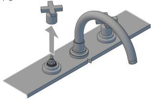
Remove the cartridge with a smooth jawed 17mm shifter.
