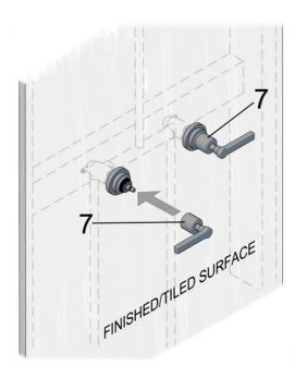
Position the retaining flange 7 with handle, over the cartridge shaft spline, and carefully hand turn the retaining flange onto thread until it is firmly seated.
