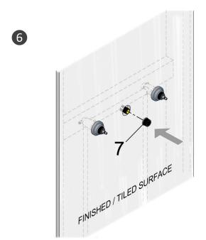
■ Fit the supplied ¾" to ½"adptor 7, into the thread section of the wall breech. Ensure it is properly sealed using PTFE tape or equivalent sealer to prevent any leakage.
