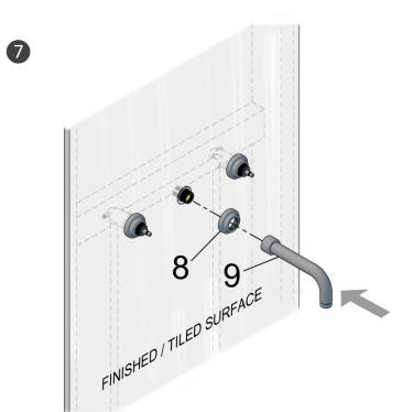
Place the cover plate 8, over the ¾" to ½"adptor. Line-up the thread end of the spout 9, with the thread of the adaptor. Apply the spout onto the adaptor and screw on until it is firmly secured. Ensure to apply adequate PTFE tape, or a suitable sealing material to the threads to prevent any leakage from the wall spout.
