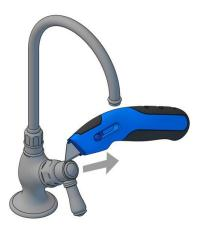
Remove the handle from the cartridge spline.
