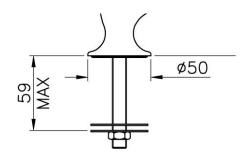
Locate the tapware in the hole of the wash basin, placing the **O-ring 1**, between the tap section base and the upper surface of the wash basin.
