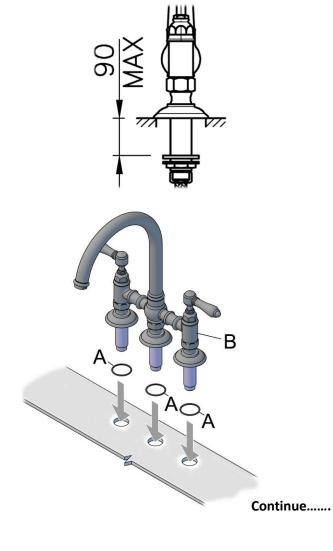
Under the sink, place the supplied rubber gaskets
