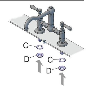
Tighten each nut using a suitable size spanner or smooth jaw shifter.
