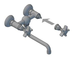
**Note:** Do not over tighten as this could damage the ceramic cartridge!
